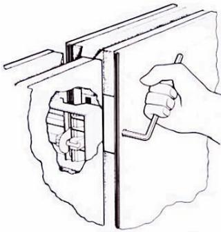
Eden Grow Room units are constructed with 4" high density foam insulation laminated between two sheets of painted galvanized 26 gauge steel creating modular insulated panels. Each unit comes with tongue and groove edged
